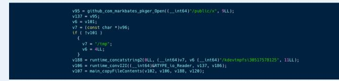
Next, it's written to /tmp under the name kdevtmpfsi, which is obviously the cryptominer, so in the older version of kinsing the malware contained an embedded version of the cryptominer that was used.
